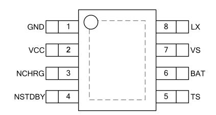
Figure 4. SLM6500 Package
